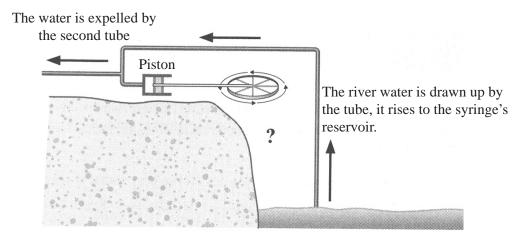
Here, the wheel is not vertical, (see the two preceding illustrations), but horizontal. In the same way as in the preceding example, the movement of the wheel's rotation makes the coming and going movement of the piston. It is now necessary to add a second wheel, this time vertical. This is what will drive the horizontal wheel due to the current of the river.
