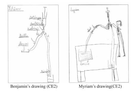
The device therefore works in two stages. First, the water is drawn up into the reservoir of the syringe by suction (1 and 2 in the below schema) via a first tube. The tap  $R^1$  is open,  $R^2$  is closed. You close  $R^1$ , and open  $R^2$ , then you push the piston of the syringe (3) in a way to expel the water to the intended place (4).
