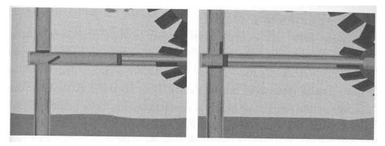
This animation extract shows the piston rotating by the slider crank mechanism. When the rod moves backward (left drawing), the first valve opens and lets the water from the river flow in by way of suction. The forward movement of the rod pushes back the piston, causing the valve to close (Right drawing). The water is then pushed backwards, leading the second valve to open, causing the water to flow upwards into the upper pipe, under the pressure of the piston.
