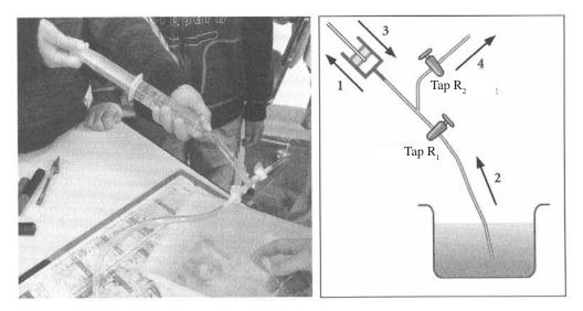
At the end of this activity, the pupils understand that the drawn water depends on the coming and going movement made by the piston of the syringe. We still have to find the means to do this without human intervention.
